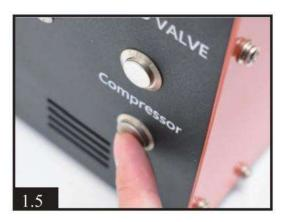
ATTENTION! Always run the fan cooling first before starting compressor.
