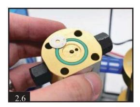
7) Loosen the 4 pieces screws on the low- pressure cylinder.
