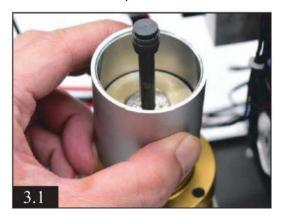
1) Setting the low-pressure cylinder into the high-pressure piston.
