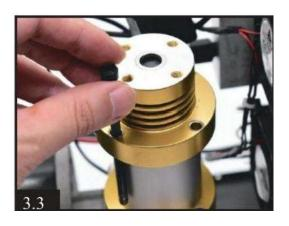
3) Setting the high-pressure cylinder into the low-pressure piston. And tighten the 4 screws.
