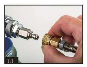
2) Connect another end foster to the output on the front of compressor via a male fitting. Make sure the foster coupling.
