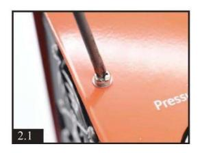
2) Loosen the one-way valve (check valve) to see if oring or spring damaged. Clean all dirt and assembly it back, which need to be tightened a bit.
