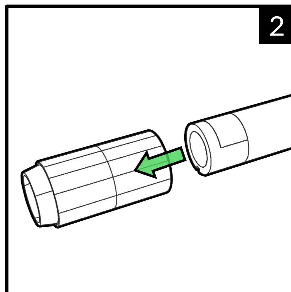
**3. First insert the inner barrel/ bucking into the hop-up chamber.**
