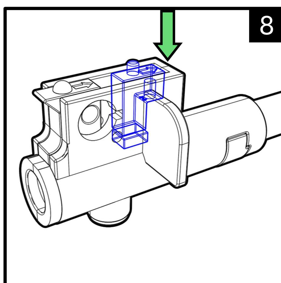
**9. Installing the hop up adjustment wheel**
