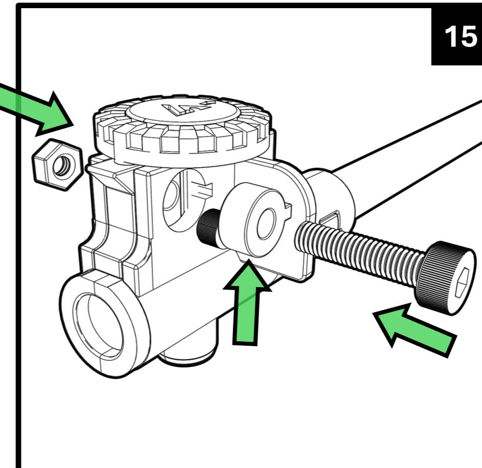
**16. Secure the M3 bolt using the nut and tighten.**
