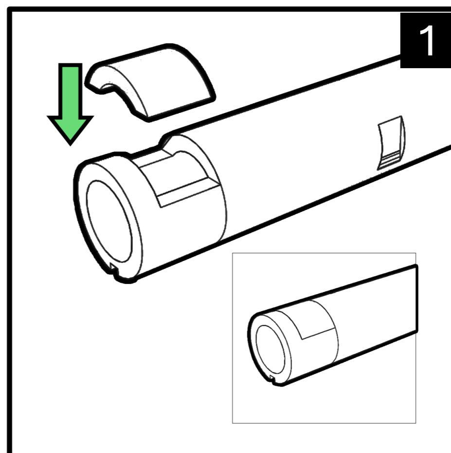
**2. Insert the inner barrel into the bucking.**
