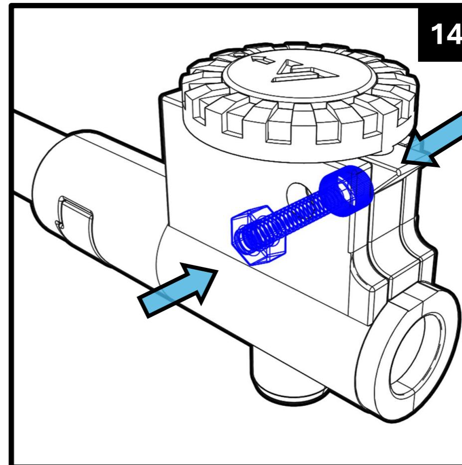
**15. M3 bolt & Nut lock, and shim**
