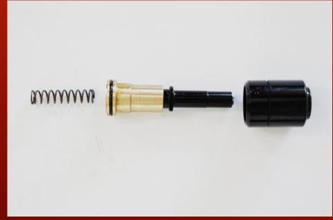
Next slide the baffle off of the nozzle/poppet assemble and pull out the spring.
