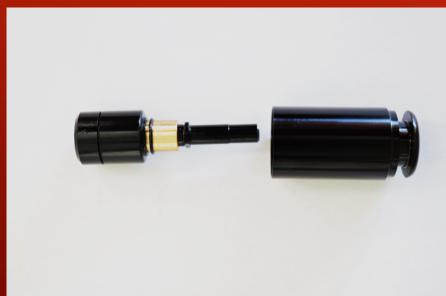
Next, disassemble the cylinder assembly by pushing the nozzle towards the back of the cylinder.
