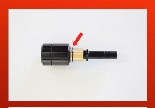
Your Inferno is ready to reassemble. Begin by sliding the poppet and nozzle assembly into the baffle. Then install the 1mm x 11mm oring around the nozzle.
